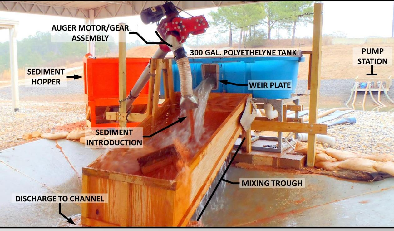
Sediment introduction is conducted using a modified grain auger. Introduction rates are regulated by controlling the auger turn velocity using a sprocket and roller chain system.
