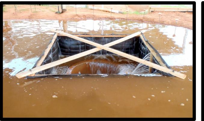
IMPROVED PRACTICE: SILT FENCE / FABRIC BARRIERS into the ground at the four corners of the installation. Flow overtopped the installation 2.5-mins into testing as a result of the imposed hydrostatic pressure. Improvements were made through Phase I procedures to develop
