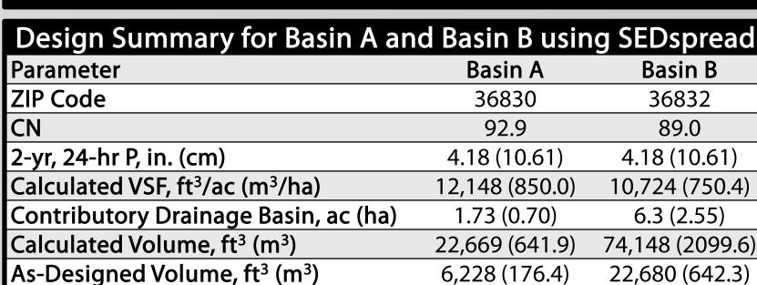
Comparing the input parameters, we see that although the projects are located in the same city, CN values differ, resulting in a VSF difference of 12% between the two sites. The calculated storage volumes for Basin A is 22,669 ft<sup>3</sup> (642 m<sup>3</sup>), which is 3.6 times larger than the originally designed containment volume. Similarly, Basin B was under designed to the 2-yr, 24-hr rainfall event by a factor of 3.3.
